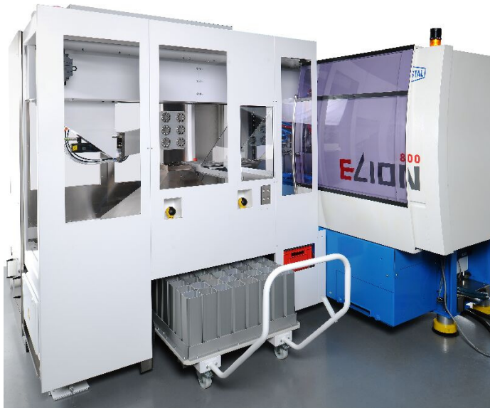
Operator's view of the compact production cell HEKUMA SI with „Sigma Inside“. Shown with a Netstal Elion 800 kN.
