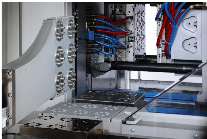
Cavity specific sorting station of the 48 needle hold end caps at the Fakuma
